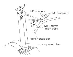
Figure 8 - Install Front Handlebar
